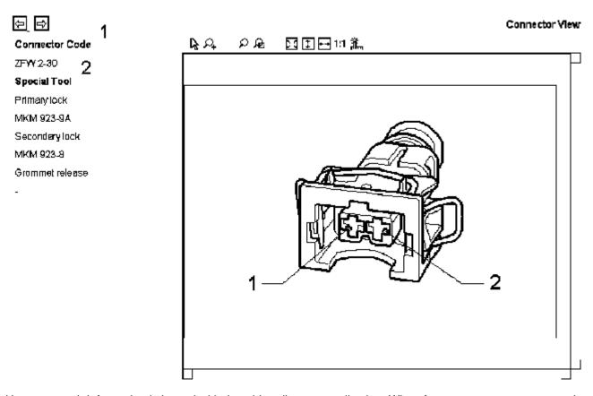
Harness repair information is issued with the wiring diagram application. When for a connector a spare part is available and repair is allowed, the text "Connector view" in the drop down box will be changed into "Connector view and repair". When with a component the text "Connector view and repair" is given, the connector code (1) and the correct special tools (2) are given with the connector view.
